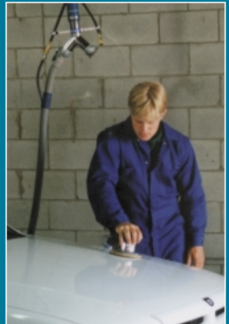
Body Shop Technician sanding car with orbital sander.
