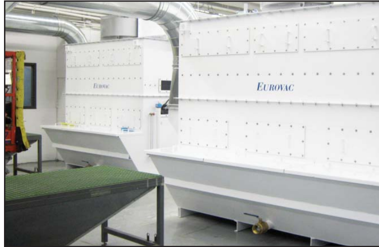
Type "A" Central Wet Collectors - Sludge Rake Dust Removal
