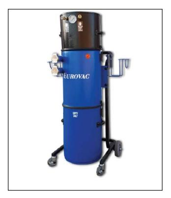
The Eurovac II portable is powered by compressed air being forced through a venturi to create a powerful vacuum. Using compressed air eliminates the chance of a dust or gas explosion as there is no sparking motor. To meet NFPA codes, the system is grounded and the vacuum hoses and cuffs are static conductive.
