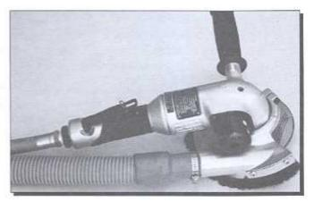
We have found that the shrouds on the market have two drawbacks. Sometimes the shroud blocks the view of the tip of the disc, particularly when using the side of the disc. The shrouds are also not totally effective in picking up sanding dust being "hurled" at 2000 to 12000 RPM off the disc. As outlined in the adjacent picture, Eurovac has a full range of retrofit shrouds. Shrouds are available for 3", 5", and 7" discs and grinding stones.
