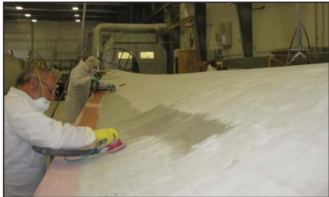
Composite wind blade turbine sanding
