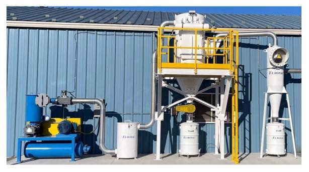
The Eurovac IV system utilizes positive displacement pumps which are available from 3 HP to 200 HP, and are capable of producing from 100 CFM to more than 3500 CFM at vacuum levels of 15" of Hg.
