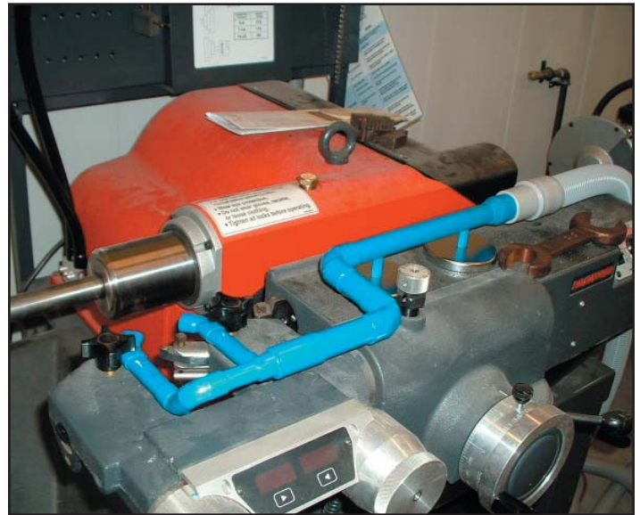
Source capture dust extraction nozzles extracting brake lathe dust back to one of the below Eurovac high vacuum systems.
