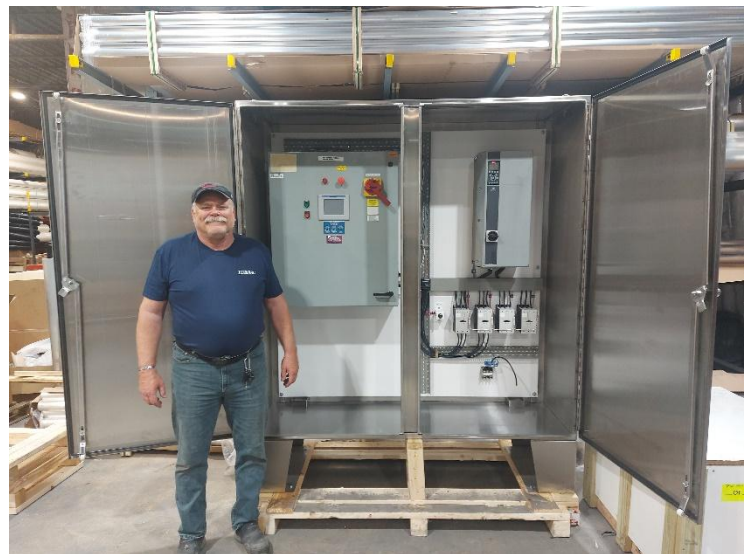
Stainless Steel Outdoor Rated Panel
